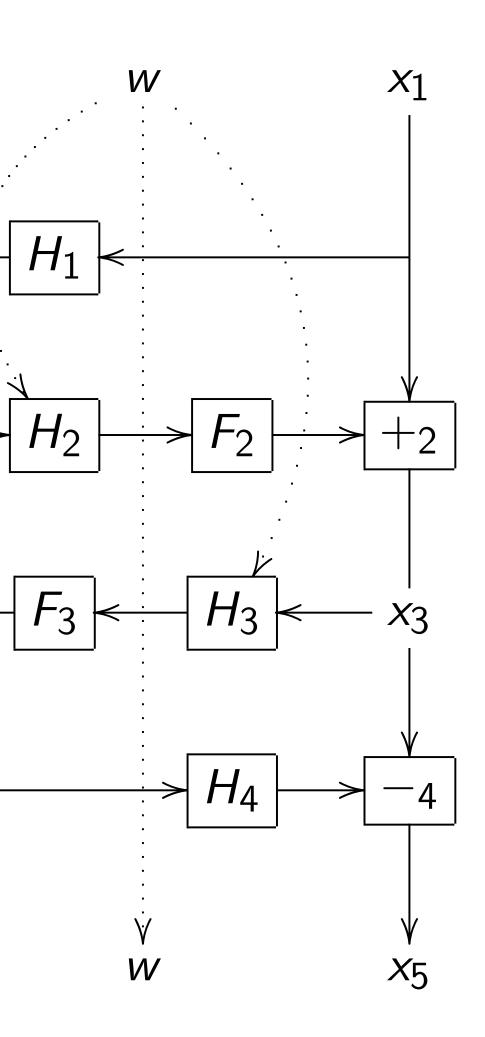
Ingredients: 4-round Feistel; H at top (1996 Lucks), bottom (1997 Naor-Reingold);  $H_2$ ,  $H_3$  allow one-block nonces;  $H_1$ ,  $H_4$  are stretched by 0-pad; XCB/HCTR-style tweak, faster than 2002 Liskov-Rivest-Wagner.
