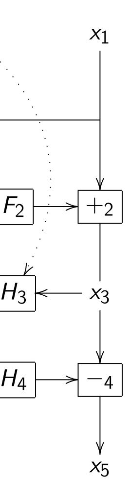
Ingredients: 4-round Feistel; H at top (1996 Lucks), bottom (1997 Naor-Reingold);  $H_2$ ,  $H_3$  allow one-block nonces;  $H_1$ ,  $H_4$  are stretched by 0-pad; XCB/HCTR-style tweak, faster than 2002 Liskov-Rivest-Wagner.
