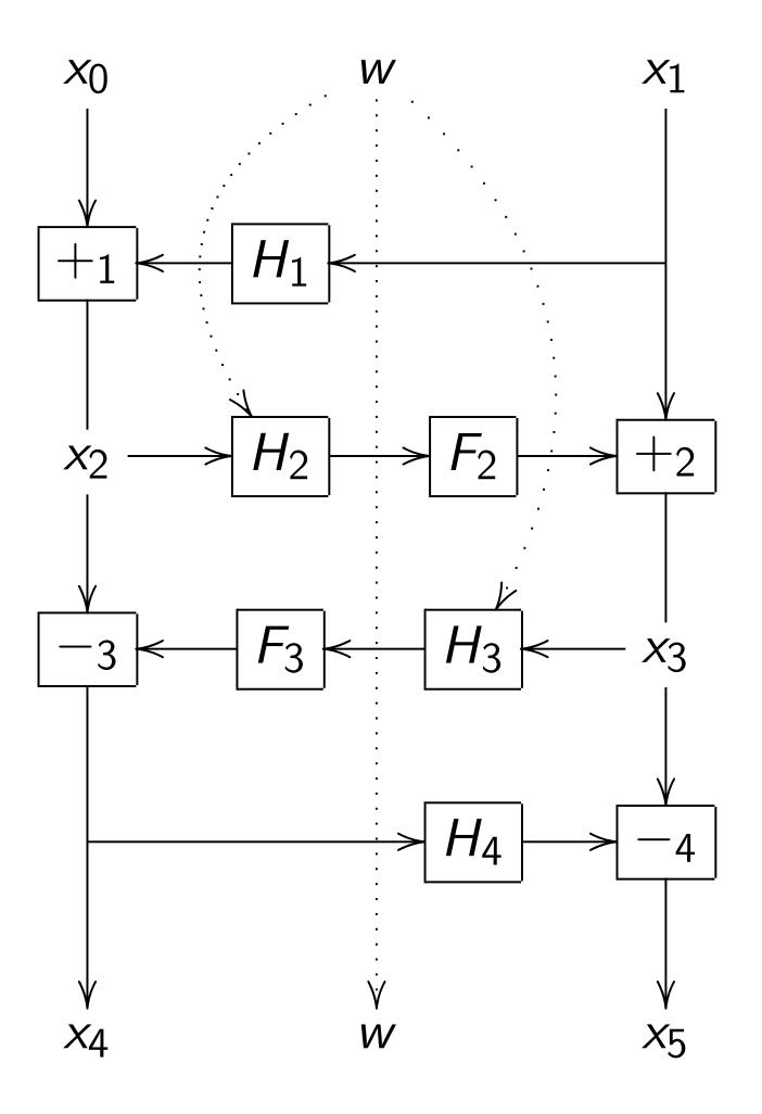
Ingredients: 4-round Feistel; H at top (1996 Lucks), bottom (1997 Naor-Reingold);  $H_2$ ,  $H_3$  allow one-block nonces;  $H_1$ ,  $H_4$  are stretched by 0-pad; XCB/HCTR-style tweak, faster than 2002 Liskov-Rivest-Wagner.
