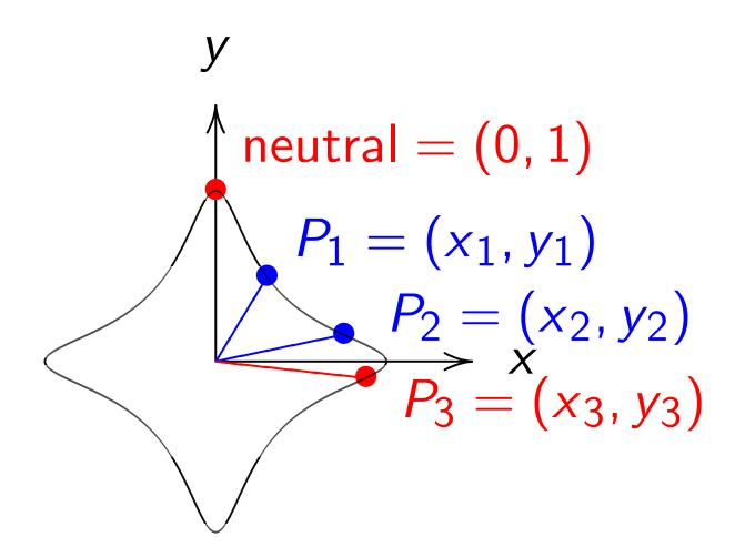
Example:  $x^2 + y^2 = 1 - 30x^2y^2$ . Sum of  $(x_1, y_1)$  and  $(x_2, y_2)$  is  $((x_1y_2+y_1x_2)/(1-30x_1x_2y_1y_2), (y_1y_2-x_1x_2)/(1+30x_1x_2y_1y_2))$ . 2007 Bernstein–La 10.8**M** for ADD, 6 ad
