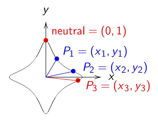
Example:  $x^2 + y^2 = 1 - 30x^2y^2$ . Sum of  $(x_1, y_1)$  and  $(x_2, y_2)$  is  $((x_1y_2+y_1x_2)/(1-30x_1x_2y_1y_2), (y_1y_2-x_1x_2)/(1+30x_1x_2y_1y_2))$ . 2007 Bernstein-Lange: 10.8**M** for ADD, 6.2**M** for DBL.
