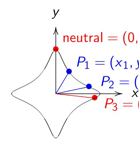
Example:  $x^2 + y^2 = 1 - 30$ . Sum of  $(x_1, y_1)$  and  $(x_2, y_2)$ .  $((x_1y_2+y_1x_2)/(1-30x_1x_2y_1)$ .  $(y_1y_2-x_1x_2)/(1+30x_1x_2y_1)$ . 1990s: ECC standards instead use short Weierstrass curves in Jacobian coordinates for "the fastest arithmetic".
