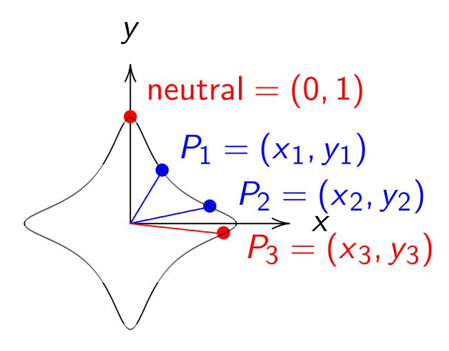
Example:  $x^2 + y^2 = 1 - 30x^2y^2$ . Sum of  $(x_1, y_1)$  and  $(x_2, y_2)$  is  $((x_1y_2+y_1x_2)/(1-30x_1x_2y_1y_2), (y_1y_2-x_1x_2)/(1+30x_1x_2y_1y_2))$ . 2007 Be 10.8**M** f ards instead ass curves nates ithmetic".
