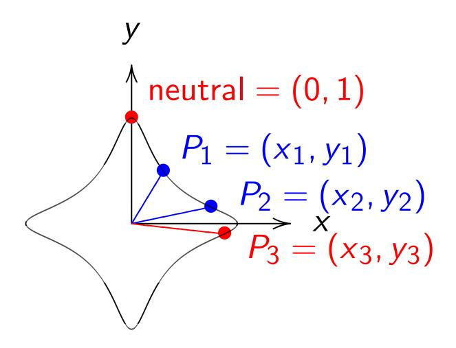
Example:  $x^2 + y^2 = 1 - 30x^2y^2$ . Sum of  $(x_1, y_1)$  and  $(x_2, y_2)$  is  $((x_1y_2+y_1x_2)/(1-30x_1x_2y_1y_2), (y_1y_2-x_1x_2)/(1+30x_1x_2y_1y_2))$ . 2007 Bernstein-Lange: 10.8**M** for ADD, 6.2**M** for DBL.
