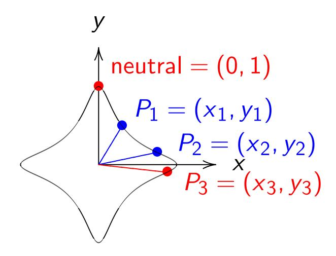
Example:  $x^2 + y^2 = 1 - 30x^2y^2$ . Sum of  $(x_1, y_1)$  and  $(x_2, y_2)$  is  $((x_1y_2+y_1x_2)/(1-30x_1x_2y_1y_2), (y_1y_2-x_1x_2)/(1+30x_1x_2y_1y_2))$ . ECC standards instead to Weierstrass curves ian coordinates fastest arithmetic".
