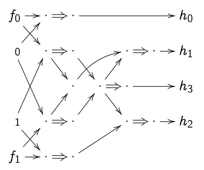
Each  $\cdot$  is a "gate"  $a, b \mapsto 1 - ab$ . This "circuit" computes product  $h_0 + 2h_1 + 4h_2 + 8h_3$  of  $f_0 + 2f_1$ ,  $0 + 2 = \mathbf{Z}$ . "Bit complexity" 15: 15 gates.
