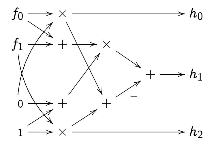
This "**R**-algebraic algorithm" computes product  $h_0 + h_1 x + h_2 x^2$  of  $f_0 + f_1 x$ ,  $_0 + _1 x \in \mathbf{R}[x]$ . "Total **R**-complexity" 7: 3 mults, 4 adds/subs.
