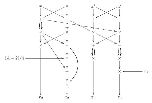
One can see at a glance that there are 4 squarings, 1 multiplication by (A-2)/4, and 5 other multiplications; and that there are 8 additions/subtractions, none of which produce input to another addition/subtraction.
